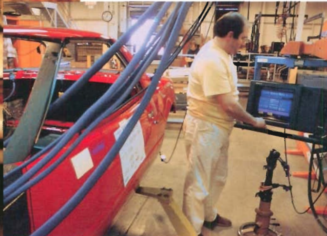
Craftsmen load customized electronic features into each Reatta via blue electrical "harnesses" which are linked to an HP 1000 A600 computer.
